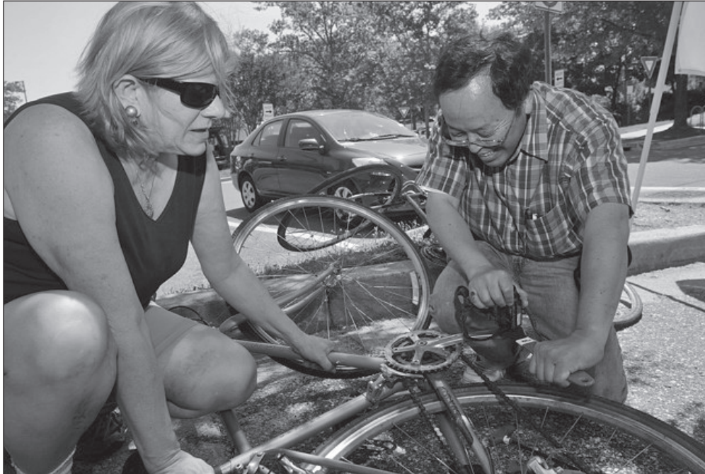
With Joy Allchin's help, Robert Yang unscrews a pedal using a pedal wrench. The pedals are then tied to the crossbar using a plastic zip tie, making them easier to store and transport.
