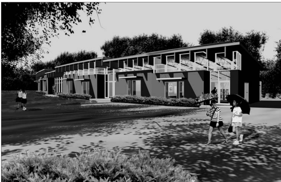
An architectural rendering of the new Friends Community School shows off the environmentally-friendly features that are planned, including straw-bale construction, a "green" roof and radiant floors.
