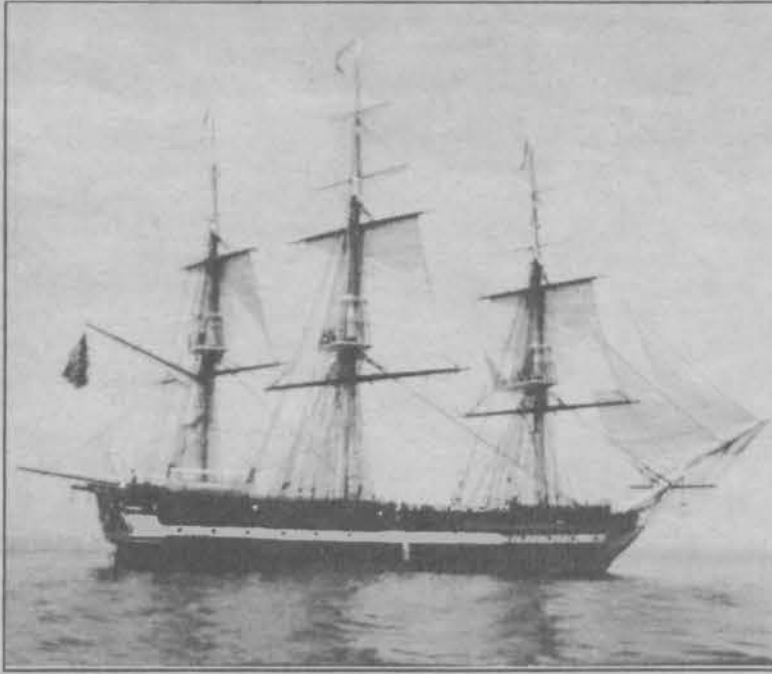
The U.S.S. Constitution, with Greenbelter John Wehrle aboard, sets sail in Boston harbor on July 8. The photo was taken from the tug Vincent. The ship is rigged with only six sails; two jibs; fore, main, and mizzen topsails. The spanker, while rigged just forward of the flag, has not yet been set. These sails are the ones used in battle with the British ship Guerriere in the War of 1812. - photo by Ken Carter
