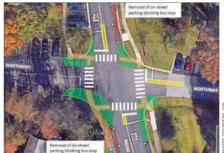
Proposed improvements to the intersection of Ridge Road and Northway. The green shaded areas show the previous design. The red shaded areas indicate sidewalks/ramps. The light gray area shows the driveway reconstruction.
