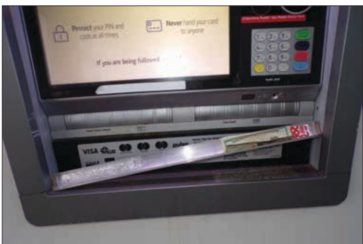
The ATM at the Bank of America on Ora Glen Drive with a device that had been covering the money slot
